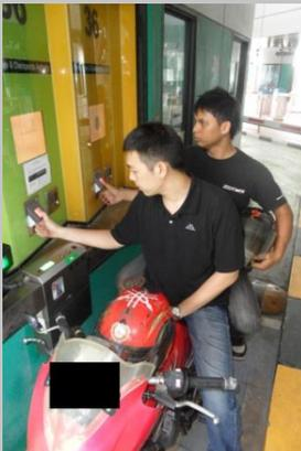
The Biometric Identification of Motorbikers System (BIKES) automates the immigration clearance of motorcyclists at the Woodlands and Tuas checkpoints. The system will authenticate the motorcyclist's fingerprint and once this is successful, the automated gate will open for the motorcyclist to pass through.
