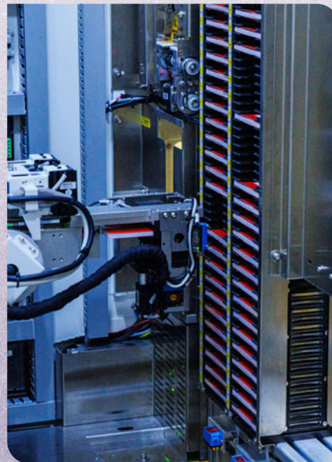
iSMART features iRobo transport robots, automated storage shelves managed by robotic arms, and self-collection kiosks
