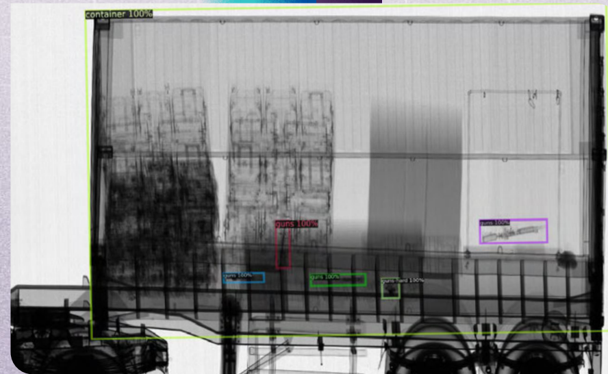
Automated AI trials successfully detect stowaways and firearms during containerised cargo screening
