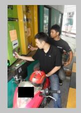
The Biometric Identification of Motorbikers System (BIKES) automates the immigration clearance of motorcyclists at the Woodlands and Tuas checkpoints. The system will authenticate the motorcyclist's fingerprint and once this is successful, the automated gate will open for the motorcyclist to pass through.
